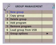
Once selected, a dialog box with the text "Create a new group" will be displayed, and in blue colour the text "Write the name". Push the rotating key or the "enter" key to begin the edition.
