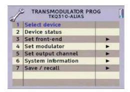
In order to program the transmodulators we need a DB9 male - RJ-45 cable (Reference: CPR 1, Code 3002026).
