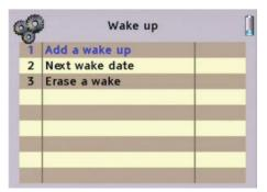
1. Add a wake up: In this option, you can create new alarms of activation of the meter. You can select date and time of power on, as well as the action to be carried out when it powers on (Datalogger or no action).
