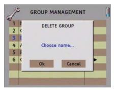
Once the option is selected, a dialog box will appear with the text "Delete Group" and in blue colour the text "Select name". Press the rotating key or the enter button to select the group you want to delete.
