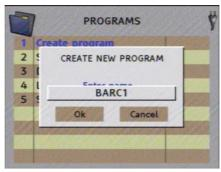
If selected signal is digital, the meter will propose the name of the program based on first current program of digital transponder/multiplex. Anyhow, it's possible to change it usging left arrow key.
