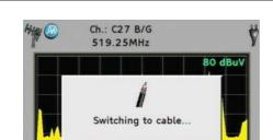
Once this option has been selected, a cable logo appears on the left top of the status bar. In case of the meter doesn't show the above message, it could be necessary to go into the "setup" menu, select "RF" option and active "show cable band".
