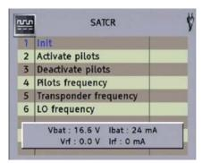
The option "Init" forces the starting of the identification of performance of the LNB previously explained.
