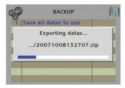
Note: if the .zip file is decompressed, the different files will be classified in different folders depending on the type of file (extension). In this manner, the backup file is organized on Programs, Datalogger, Satellites or Autoscan.
