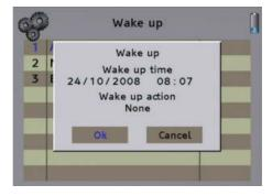
2. Next wake date: In this option, the next alarm will be shown, being able to see the day, time and action to do in the activation of the meter. If no alarm is created, one alert will be shown in the screen.
