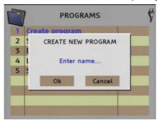
If analog signal is selected, the name of the program should be completely wirtten. To enter letters and numbers, press "abc/123" key for alphanumerics. It's possible to delete wrong letters using left arrow key.
