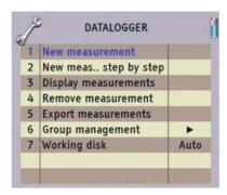
Once it is selected, a dialog box will appear with the text "New measurement". In the field "Add measurement to the group" select the name of the group where you want to store the measurement.
