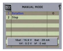
The **Rotation** value indicates the number of motor steps to be turned, towards East if the value is positive, or towards West if it is negative. In our motor **DiMo 120**, each step of the motor is equivalent to a 1/10 of degree.
