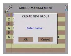
To name the group, please introduce it with the alphanumeric keys of the keyboard. In case of error, it is possible to delete the last setter by pressing the left arrow of the horizontal cursors. Once the name has been written, please push **enter** and turn the rotating key to right to select "Yes" and confirm to store it.
