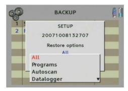
Pushing on the backup, a dialog box opens with the list of available files to be restored:
