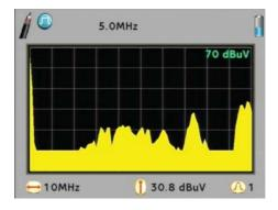
3.- "meter" key active. The monitor is divided in two parts: status bar and signal measurements information.
