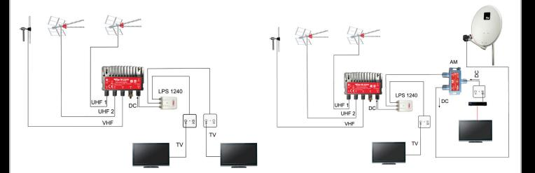
The LPS 1240 power supply allows current to pass from the output to the input. Do not introduce a voltage through the outputs of the source when using this mast amplifier since it should only be fed at 12Vdc. You can use two DCBs on the source outputs to block any DC voltage.
