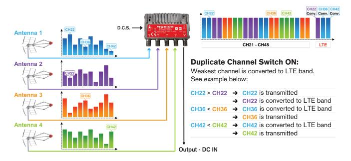
ON- Reassigned Channels: When two antennas receive the same channel, the weaker channel is converted to the LTE band
