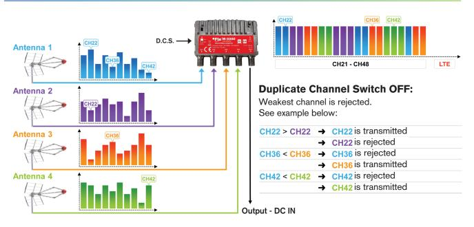
OFF- Reassigned Channels: When two antennas receive the same channel, the weaker channel is rejected
